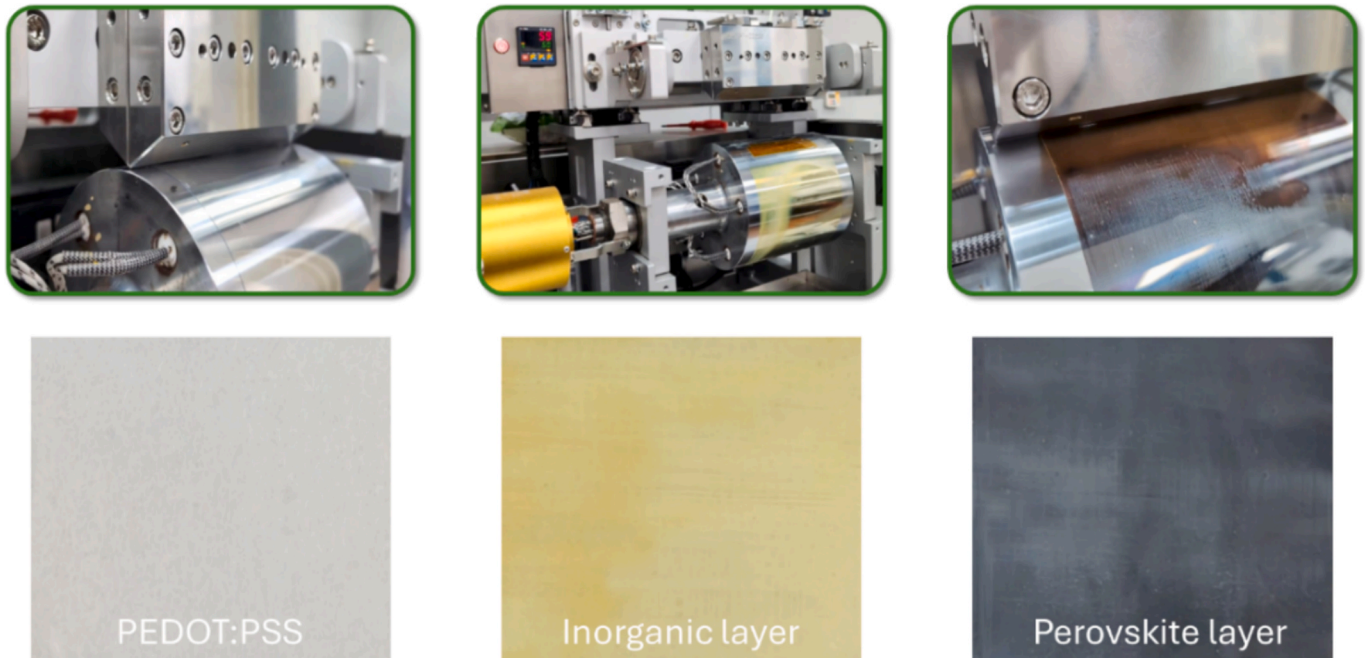
Fig. 5. The image illustrates the film layers fabricated using the R2S coating technique, including the PEDOT:PSS layer (hole transport layer), the inorganic layer, and the perovskite layer. It also shows the appearance of the completed film layers after coating, highlighting their smooth and uniform surface.
