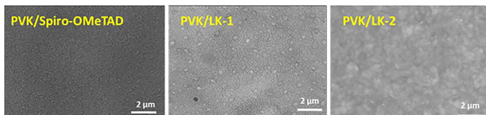
Figure 4. Top-view SEM images of PVK/spiro-OMeTAD, PVK/LK-1 and PVK/LK-2.
