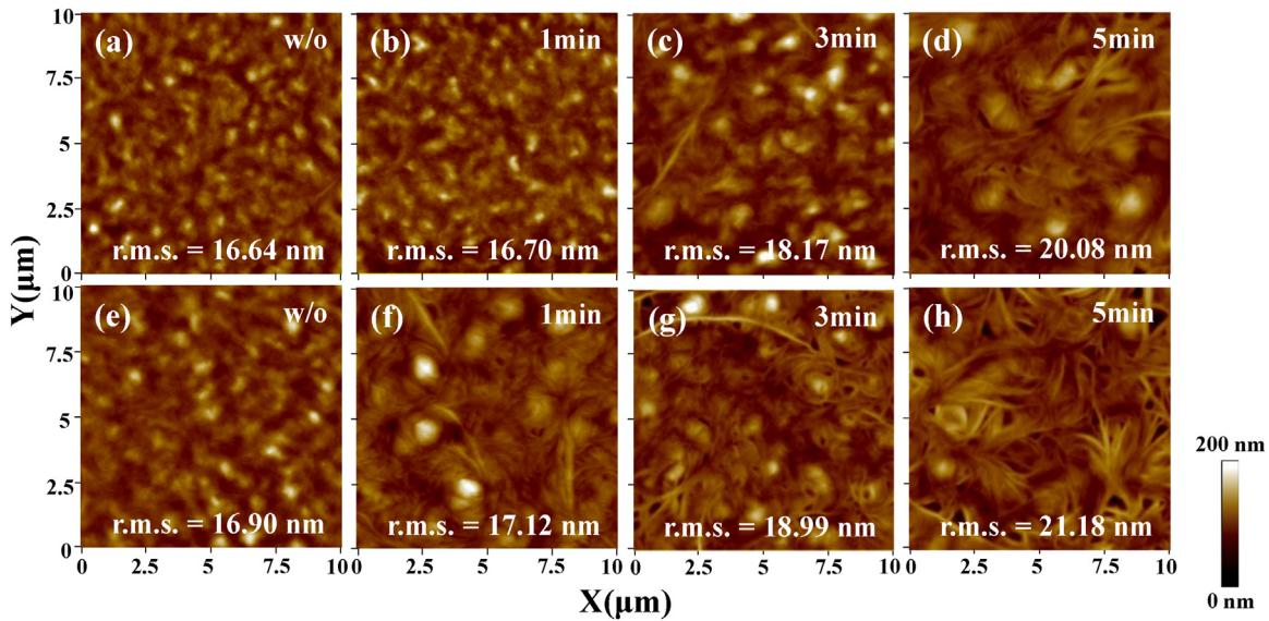
**Fig. 3.** AFM topographic images of the P(VDF-TrFE) copolymers on the (a,e) untreated and (b,f) 1-, (c,g) 3-, and (d,h) 5-min CF<sub>4</sub>-plasma-treated IGZO films before and after annealing, respectively. The surface roughness (r.m.s.) measured by topographic images was noted in these figures.
