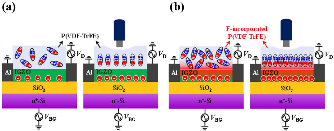
**Fig. 6.** The schematic diagrams of (a) untreated and (b)  $\text{CF}_4$ -plasma treated piezoelectric pressure sensors with IGZO TFTs coated by P(VDF-TrFE) copolymers before and after the force applied, respectively.
