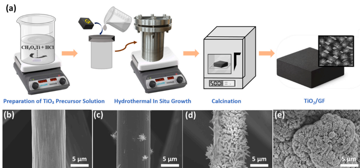
Fig. 1. (a) Schematic illustration of the in-situ hydrothermal growth process of \text{TiO}_2 nanostructures on graphite felt ( \text{TiO}_2/\text{GF} ). SEM images of (b) pristine graphite felt (GF), (c) sea-urchin-like \text{TiO}_2/\text{GF} (SU- \text{TiO}_2/\text{GF} ), (d) nano-rod-like \text{TiO}_2/\text{GF} (NR- \text{TiO}_2/\text{GF} ), and (e) nano-flora-like \text{TiO}_2/\text{GF} (NF- \text{TiO}_2/\text{GF} ).
